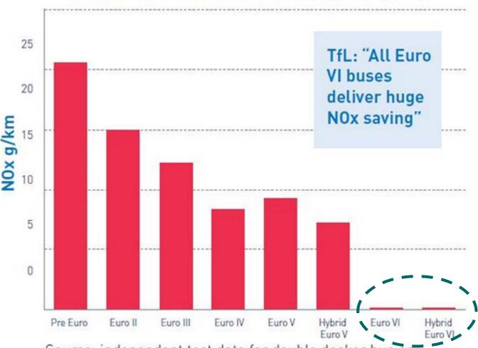
Source: independent test data for double decker bus on London 159 test route
